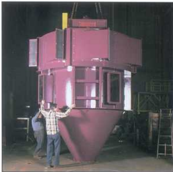
SD fit being checked prior to shipment
