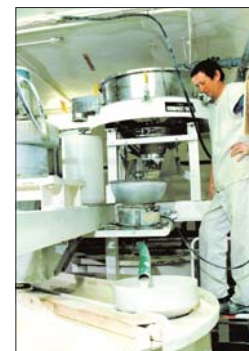
Compact Sieves are suitable for screening wet materials as shown here at Royal Crown Derby.
