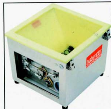
Paddle Drive Adjustable Linkage Easily Accessible From Rear of Feeder
