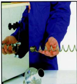
STEP 1 - Remove the screw tube (3 bolts) and screw (threaded connection).
