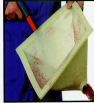
STEP 4 - Washing the polyurethane hopper, if necessary.
