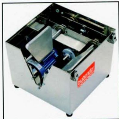
Massaging Paddles, Motor and Screw Connection
