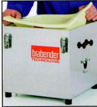
STEP 3 - If necessary, remove the flexible polyurethane hopper by simply pulling the sealing lip off the upper edge of the housing for further dry cleaning or washing.
