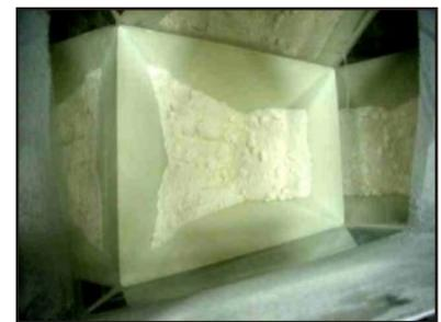
The trapezoid shape and paddle activation pushes the ingredient toward the lead screw flight. The ingredient level in the hopper remains flat.
