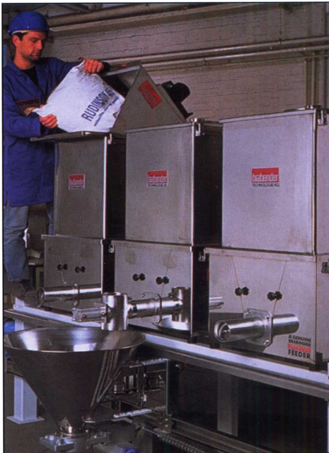
A three feeder BatchMaster Feeding Station with pneumatic shut-off valve on center feeder. Operator empties bag into Brabender Bag Dump Station.
