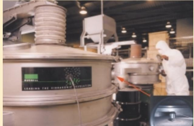
An ultrasonic deblinding system being used to help sieve metal powders at Mining and Chemical Products Ltd., Northamptonshire, UK.
