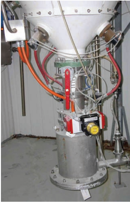
The 1-cubic-foot-capacity Mini-Jet, which is mounted directly beneath the bulk silo, can convey up to 1,000 pounds of salt per hour.
