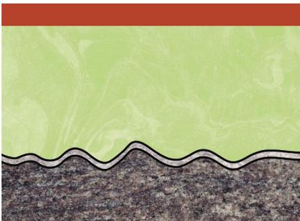
Figure 4. Stainless steel after electropolishing.
