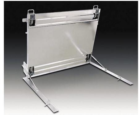
Figure 6. Pharmaline platform scale opened to 90 degrees for easy cleaning below the scale. This low-profile platform scale is designed for cleanroom areas. Its AISI 304 electropolished construction, rounded corners, and integrated pressure-lift system satisfies basic cleanroom needs.
