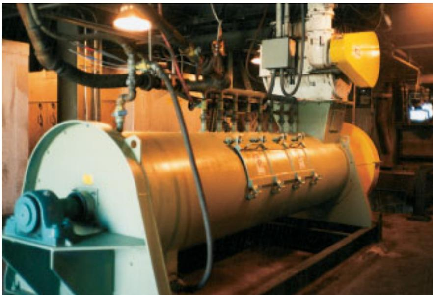
*The rotary airlock (upper right) feeds 70 to 80 tons of fly ash per hour into the blending chamber, where moisture is added for dedusting.*
