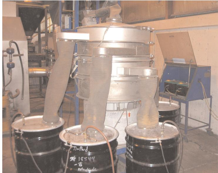
The Russell Vibrasonic Deblinding System being used at the Reading Alloy plant, with their existing screener
